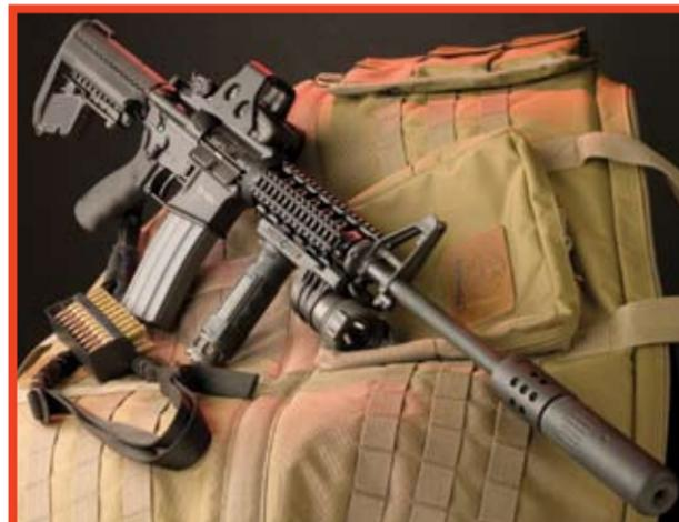
AAC Omni Suppressor fits over standard "birdcage" flash suppressor without adapters and significantly reduces muzzle blast and flash. Suppressors are considered essential by many tactical teams for clearing buildings where muzzle blast is amplified by interior walls, reducing ability of team members to effectively communicate.
